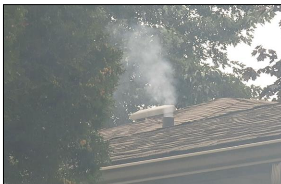
Smoke out of plumbing vent and internal plumbing indicating a connection with storm sewer.
