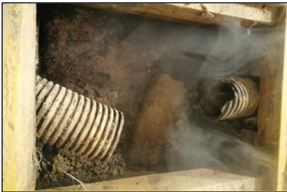
Smoke out of sump pit / cleanout in the basement indicating a connection with the storm sewer via foundation drain and storm lateral.
