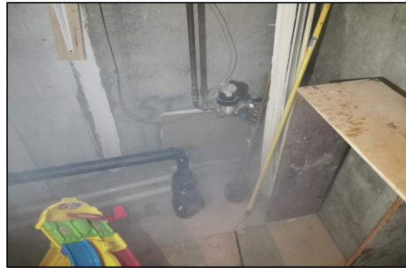
Smoke out of sump pit / cleanout in the basement indicating a connection with the storm sewer via foundation drain and storm lateral.
