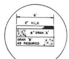
TYPICAL X SECTION PEDESTRIAN FOOTPATH N.T.S.
