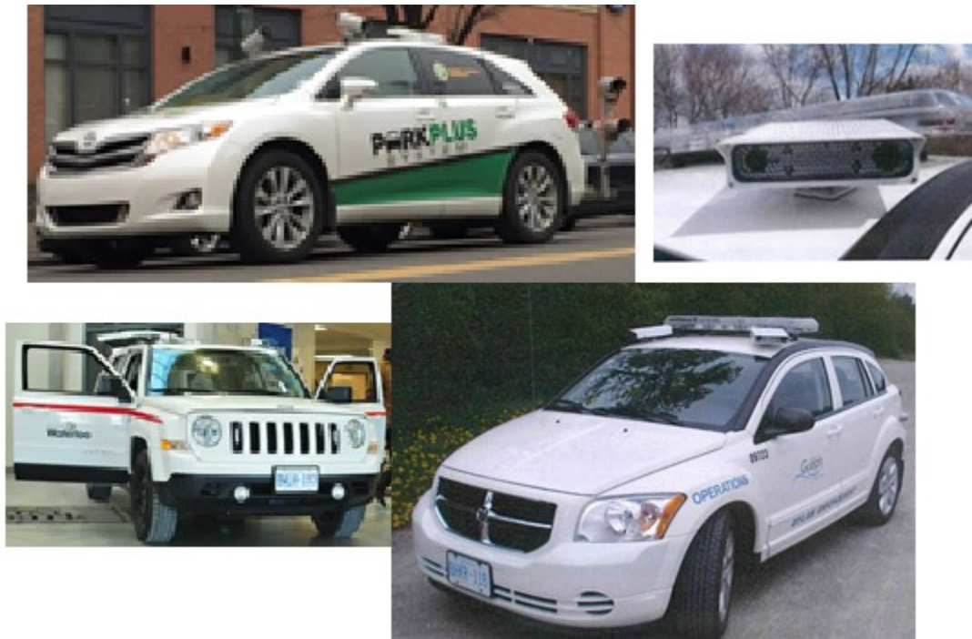
Figure 16 - Mobile Parking Enforcement using Licence Plate Recognition (LPR) in Calgary (top left), Waterloo (left) & Guelph (right)
