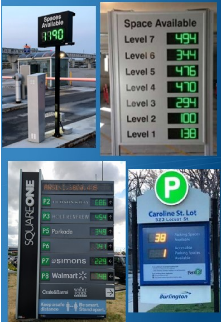
Figure 32 - Digital Parking Space Availability Signs at Entry Points
