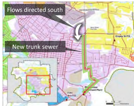
Alternative 1B: Existing Flow Split with New Downtown Trunk Sewer to Wastewater Treatment Plant
