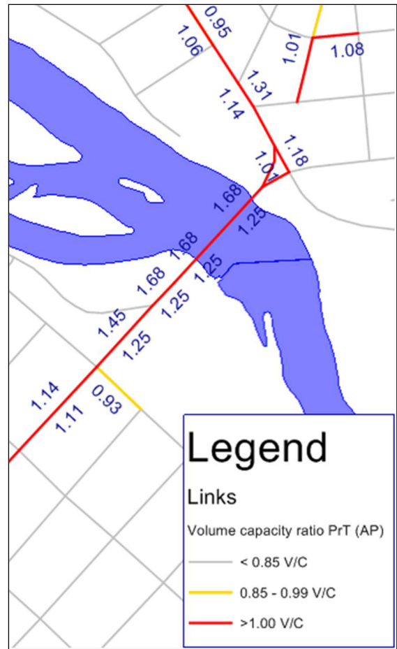
Figure 4-29: Colborne Street (Lorne Bridge) – Crossing the Grand River: 2041 PM Peak Hour V/C Ratios
