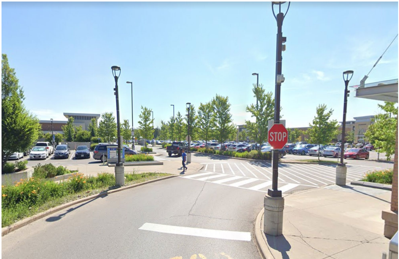
Surface parking and pathway orientation should be arranged to delineate clear pedestrian pathways, vehicle routes, and accessible parking, and accommodate landscaping, lighting, physical separations and painted lines / Markham, ON.
