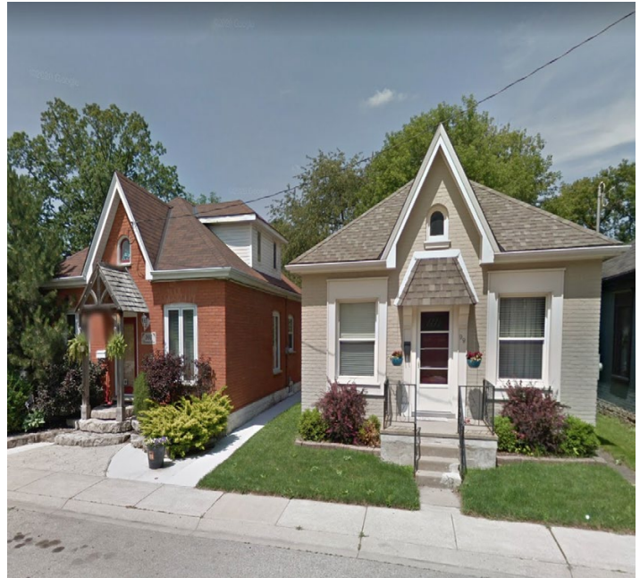
Front entrances should front the street and be fully visible, located at grade or at height of approximately 1.5 metres above grade / Chestnut Ave.
