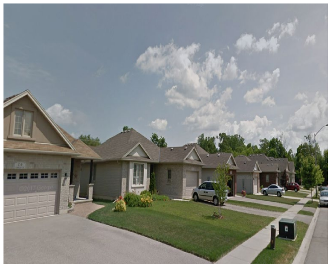
Controlled front yard setback variation provides visual interest on straight street blocks / Jamieson Ct.
