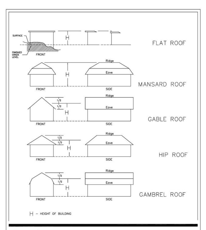
Figure 2.1 Illustration of BUILDING HEIGHT DEFINITIONS
