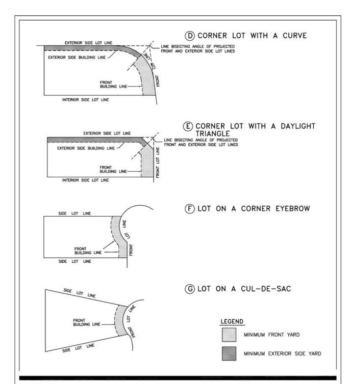
Figure 2.4b Illustration of MINIMUM FRONT YARD and MINIMUM EXTERIOR SIDE YARD City of Brantford Zoning By-Law
