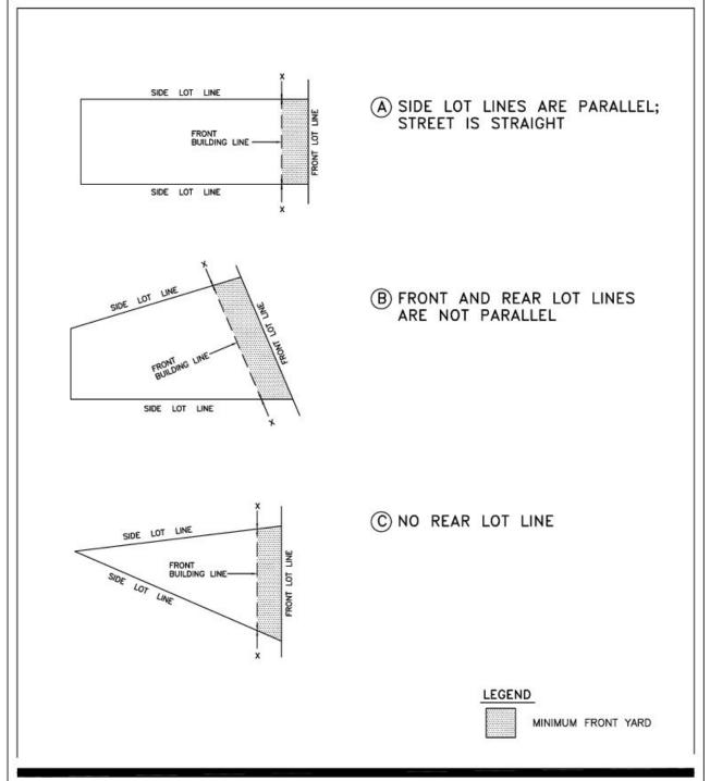
Figure 2.4a Illustration of MINIMUM FRONT YARD and MINIMUM EXTERIOR SIDE YARD City of Brantford Zoning By—Law
