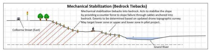
Figure 5-2. Alternative Design Concepts in Profile for Mechanical Stabilization
