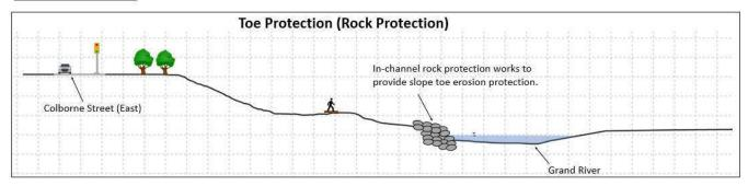
Figure 5-1. Alternative Concepts in Profile for Toe Protection
