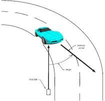
Figure 5.2.1 An angle between the antenna and the target vehicle causes the cosine effect.
