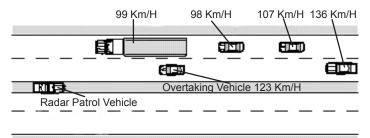
Figure 3.5 The vehicle going 123 kph is the next strongest target going faster than the strongest.
