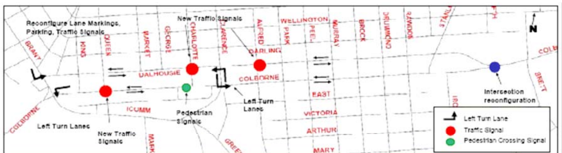
Exhibit 4.1: Proposed Improvements to Support One-way Street Conversion
