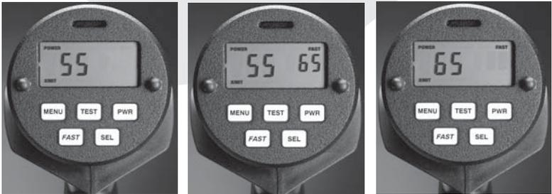
Figure 3.5.2 Strongest Signal, Faster-Toggle, and Faster-Hold modes
