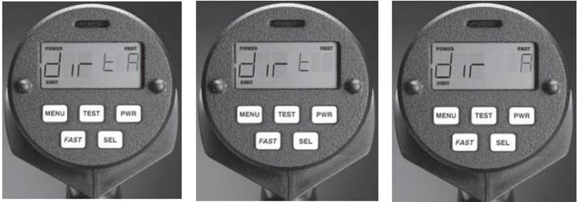
Figure 3.3b The dir option displays tA, t or A.
