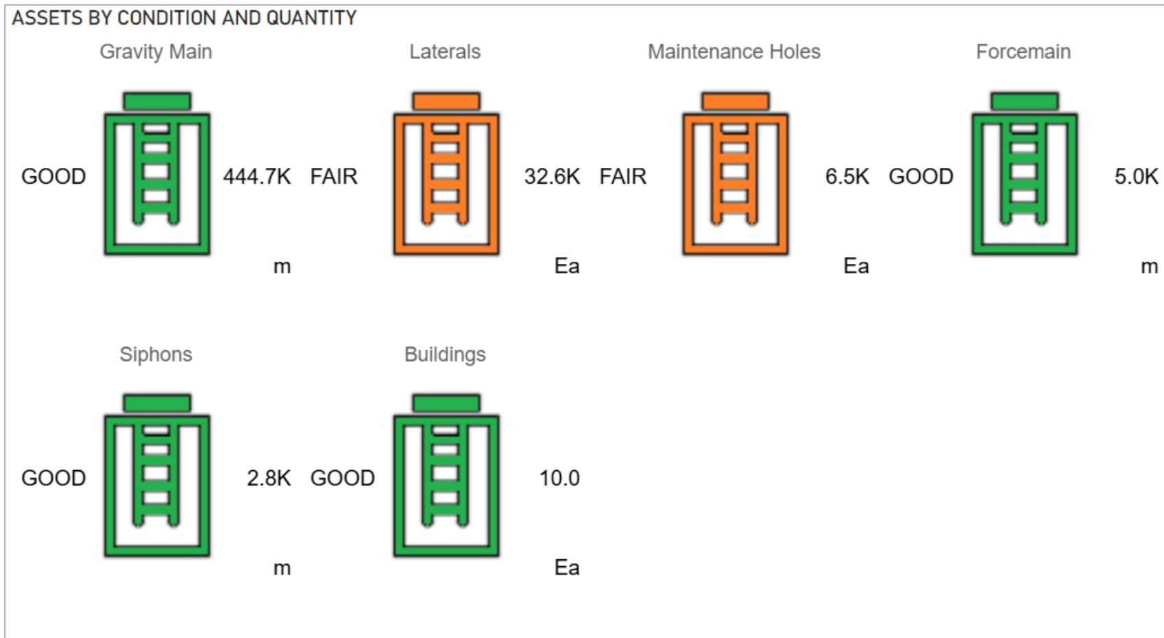
Figure 4 Wastewater Collection Asset Summary by Condition and Quantity
