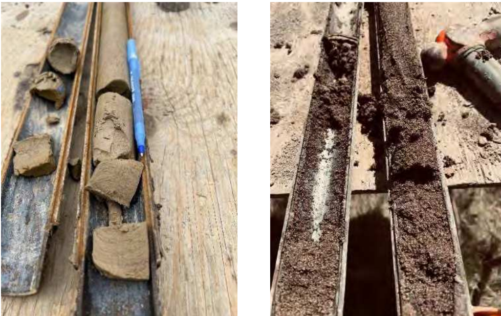
Figure 3.20: Fractures in silt/silt clay matrix filled with fine sand at MW-1 (left) and coarse sand encountered at MW2-D (right).
